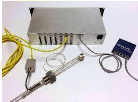
Oscillator Box with Cables and Feedthrough
