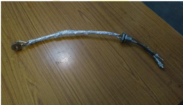
Water Cooled Crystal Holder with Feedthrough and BNC Cable
