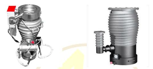
Diffusion Pump is an oil based vacuum pump used for obtaining high vacuum  $< 10^{-6}$  mbar with suitable capacity backing pump. It is operated with oil of low vapor pressure.
